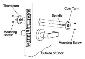
III. Fasten inside thumbturn by two (2) mounting screws, and fix coin turn by provided screws on the outside face of the door.
