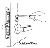
IV. In case emergent situation, use a coin or flat tip screwdriver to unlock door.
