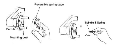
C.Install outside lever with mounting posts through door and position spindle with spring into hub of lock case.
