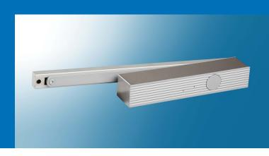
MAAX C2600 Series door closer is designed to provide higher efficiency with the aesthetics of track type door closer. The innovative cam-action design provides strong closing force and control at the latch position while offering much lower opening resistance which makes the door very easy to open. The C2600 closer is an ideal solution for large sized door openings in institutional and commercial applications including hospitals, universities and office buildings.
